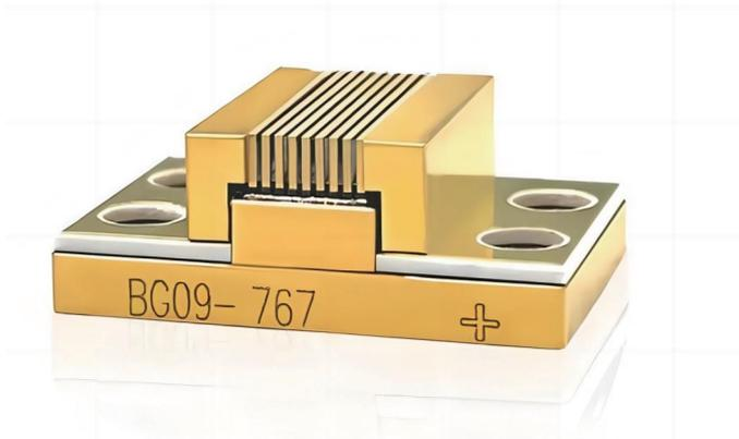
Devices that use high-power semiconductor laser bars as light-emitting components are collectively referred to as bar lasers, which are also known as array products, including components such as the laser bar, heat sink, and electrodes. The main difference from single-emitter devices is that the bar contains multiple emitters, which are electrically parallel to each other.
